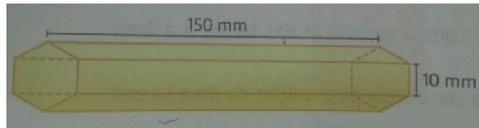
Figura 42: Prisma hexagonal regular.
